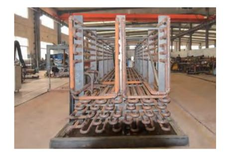
The barrel is transport to the platform by the forklift, and receiving arms turn over the bitumen barral into the melting room by hydraulic control.
