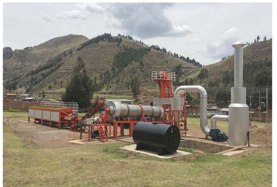
DHB80 Continuous Asphalt Mixing Plant Erected in Peru
