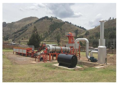
DHB80 Continuous Asphalt Mixing Plant Erected in Peru
