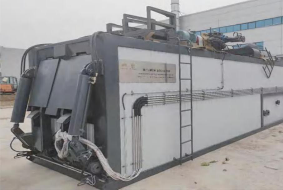
Hydraulic Drummed Bitumen Decanter in Uzbekistan
