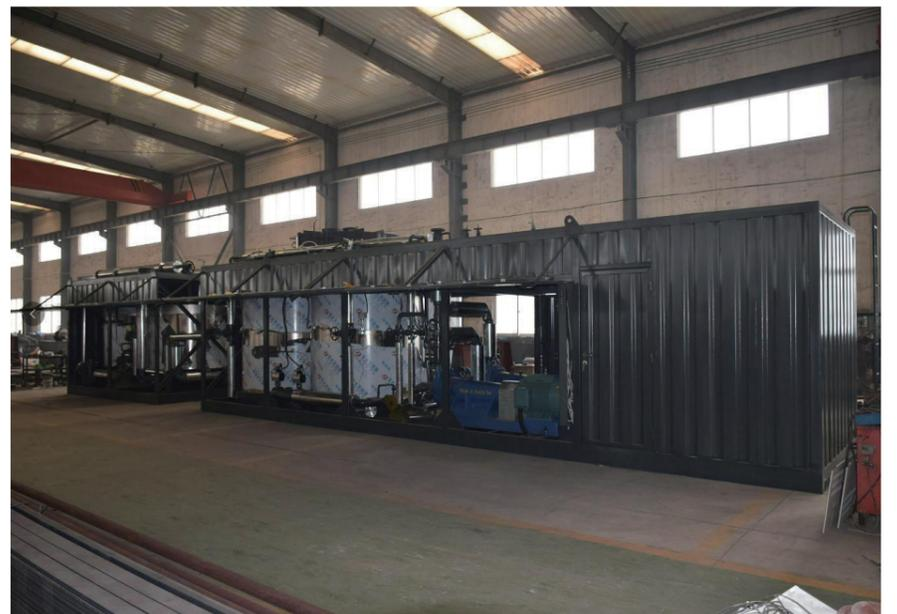
Polymer Modified Bitumen Plant in Australia
