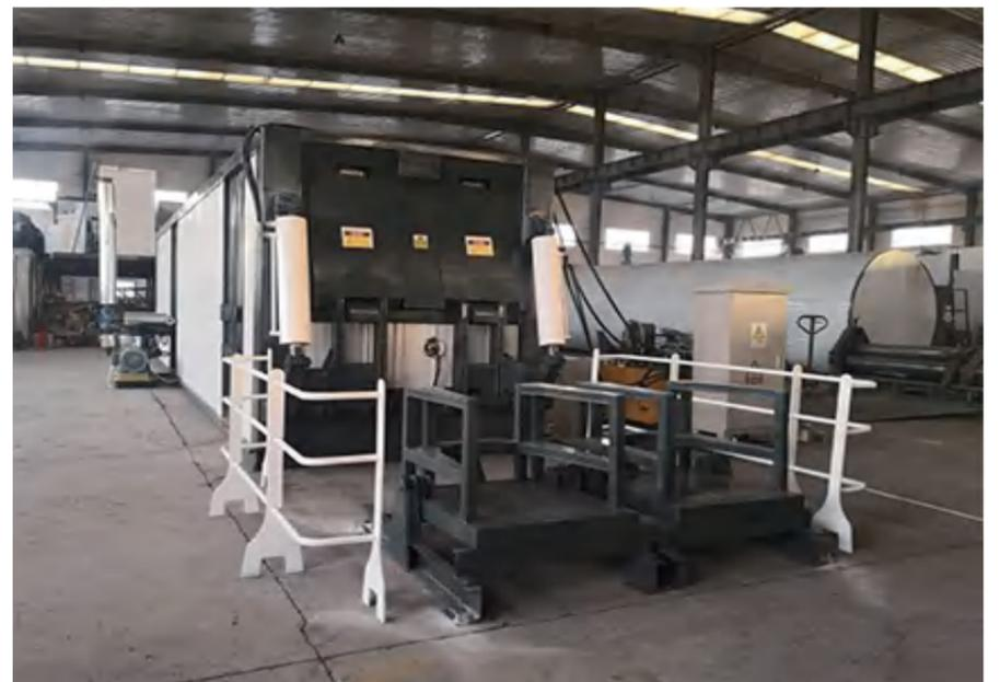
Bitumen Melting Machine/Bitumen Decanter in Africa
