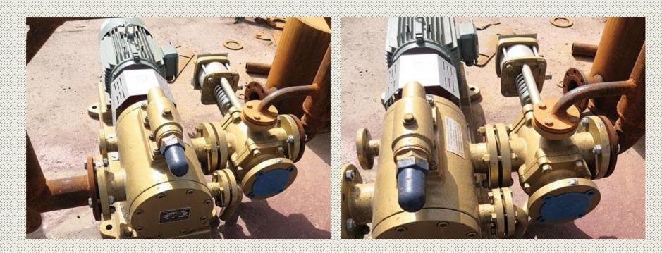
The 3QGB series heat-preservation high-viscosity three-screw pumps are mainly used to convey high-viscosity lubricating fluids. They are usually used as the delivery pumps of asphalt, heavy fuel oil, heavy gear oil and heavy diesel fuel. Inside the pumps, heat preservation chamber and channel are set us, gas or liquid could be used as heat carrier, and their maximum working temperature is equal to or lower than 350°C. High viscosity reduction, and the conveying viscosity is generally 3.0~760mm2.
