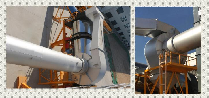
1. The system adopts high-pressure pulse cleaning method, and the residual dust is small. All the dust can be transported to the circulating silo for reuse or discharge through the recycling packing conveying device. Emission concentration does not exceed 20mglNm3
