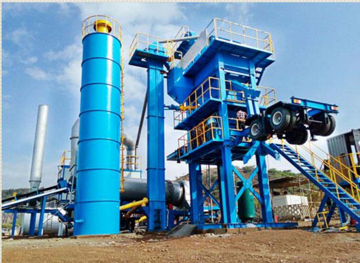
**YLB Mobile Asphalt Mixing Plant**
